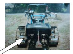
Figure 10: The arrow pointing to the tilling wheel with heavy duty blades steel linked to the connecting the central rotor and the tilling blades.
