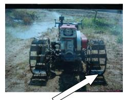
Figure 11: The arrow pointing to the steel link connecting the central rotor and the tilling wheel with heavy duty blades
