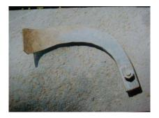
Figure 12: The steel connecting plate that was pointed in the earlier photograph is seen here. the nut has loosened and the nut side end has pierced and entered the medial aspect of the patient's thigh.
