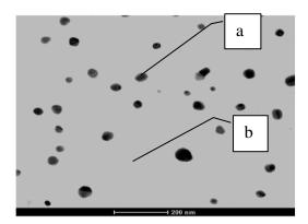
Figure 1: An electron microscope image of NPs:Ag. a – silver nanoclusters; b – amorphous carbon matrix.
