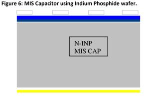
Metal Insulator semiconductor devices are used to fabricate Bio-electrodes for Medical Applications. We have fabricated the MIS capacitor device as test vehicle for MISFET device and given detailed fabrication steps.
