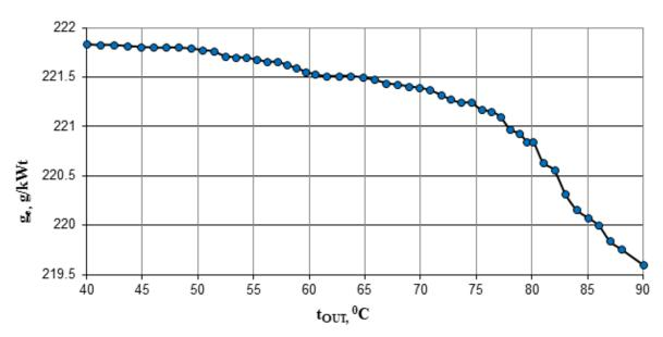
Figure 2: Dependence of specific fuel consumption on the CF temperature
