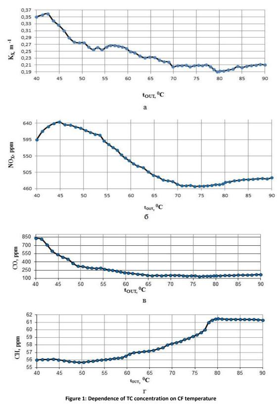
а - opacity  $K_x$ ;6 – nitrogen oxide NO<sub>x</sub>; в - carbon monoxide CO; г – carbohydrates CH
