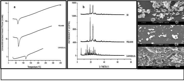
Figure 2: (a) Overlaid DSC Thermograms; (b) Overlaid diffractograms from XRPD Studies; (c) SEM Micrographs of (i) Carvedilol, (ii) PEG-6000, (iii) CAR-SD.
