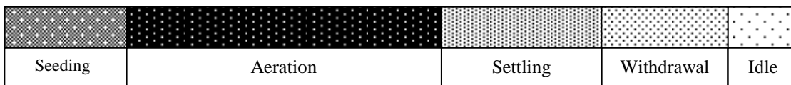
Figure 1: Dynamic process conditions of the SBR used in a successive 24-h cycle
