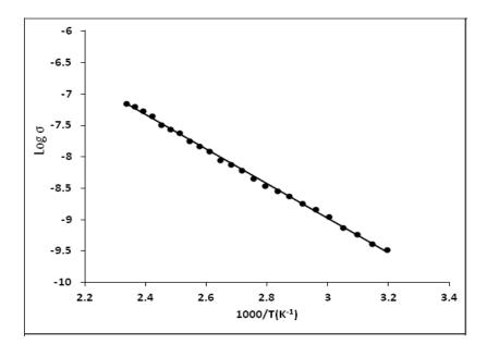
Figure 6: Electrical conductivity of 4-HACF copolymer resin
