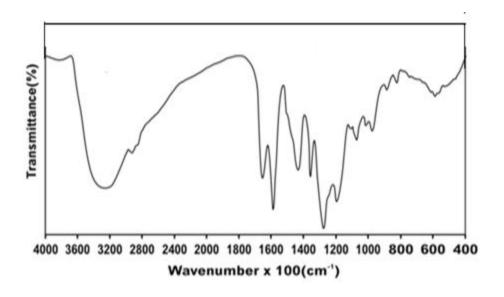
Figure 3: Infra-red spectra of 4-HACF copolymer resin
