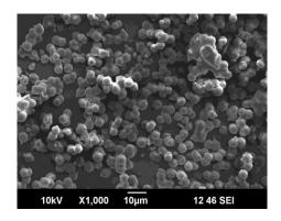
Figure 5: Scanning electron microscopy of 4-HACF copolymer resin
