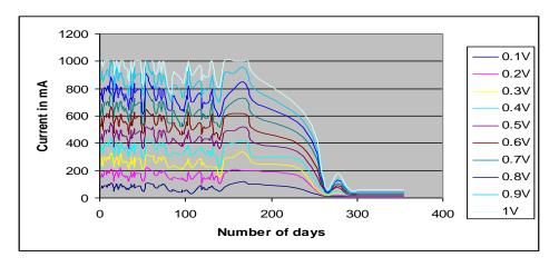
Figure 26. The variation in current as healing proceeds for 0.7 V D.C input.
