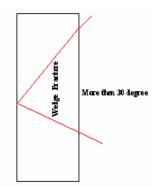
Figure 38. Wedge fracture with obliquity
