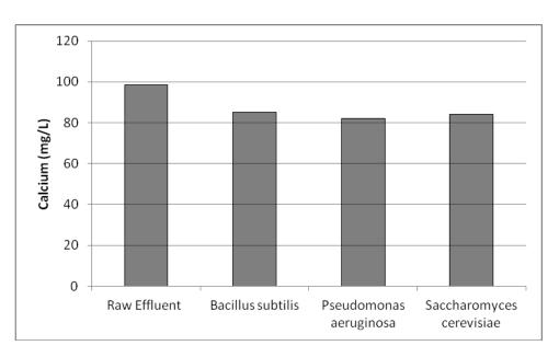
Figure 1: Application of microbes in removal of Ca from tannery wastewater
