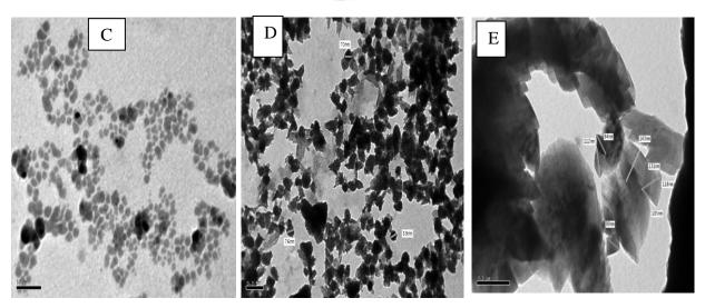
Fig. 2 (A) UV–Vis spectroscopy of zinc oxide nano particles prepared at different pHs. Reaction conditions: 2.9g/I HEC, (1.3g/I) zinc nitrate; temperature 80°C; duration 30 min., and stirring rate 150rpm (B) variation of major obtained particle size of nano zinc oxide due to variation of pH value. (C) TEM image of the sample obtained at pH 11, (D) TEM image obtained at pH 12.5, and (E) is TEM image obtained at pH 14
