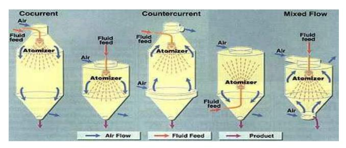
Fig.3: The atomized droplets that are formed from the atomizing device established by the atomizer
