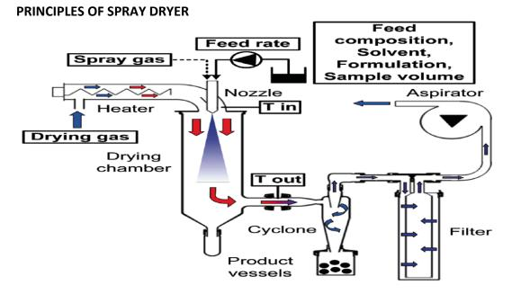
Figure 1: Process diagram of the Mini Spray Dryer B-190, B-191 and B-290 models with process parameters.
