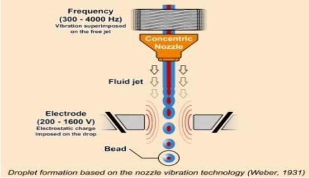
Fig 2: Droplet Formation Based On The Nozzle Vinration Technology
