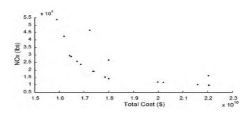
Figure 3: Tradeoff between cost and NOx [14]
