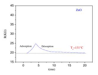
Figure IV.3: Variation of resistance with time during an adsorption - desorption of oxygen on sample of ZnO at  $T_a = 131$  ° C.
