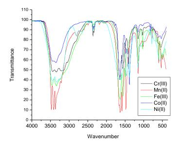
Fig. 2: Infrared spectra of urea complexes.
