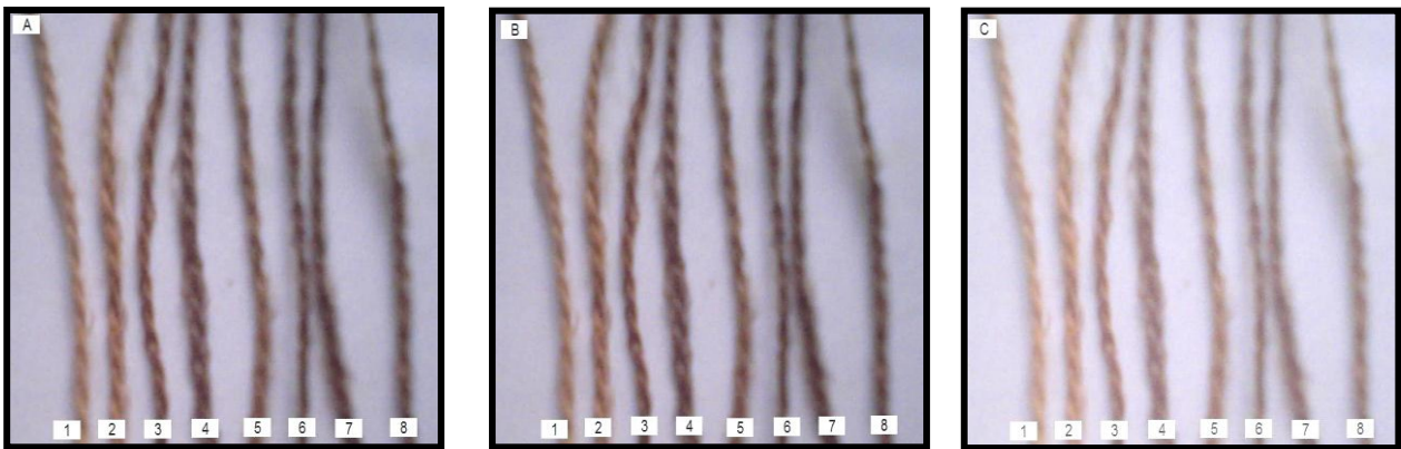
Fig. 3: Photographs of wool pieces treated with formulations containing aqueous extract on (A) zero day (B) fifteen day and (C) thirty day when detergent washed.
