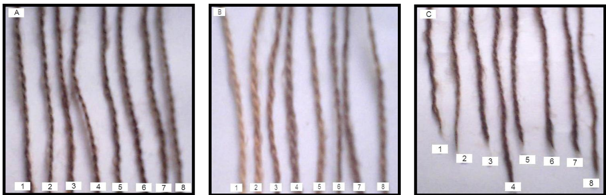
Fig. 4: Photographs of wool pieces treated with formulations containing alcoholic extract on (A) zero day (B) fifteen day and (C) thirty day at room temperature.
