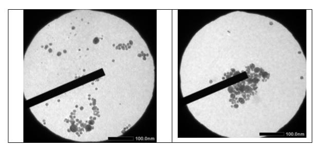
Figure 1. The clusters of gold NPs concentration 5 ppm(left) and 10 ppm(right).
