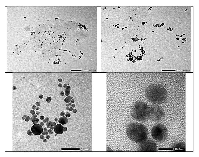
Figure 2.TEM of nanogold with several magnifications to measure diameters of clusters.
