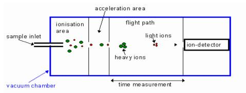
Fig 6 Mechanism of Time-of-Flight
