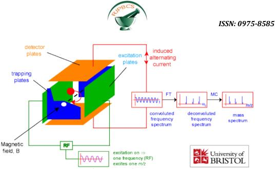
Fig 8 Mechanism of Fourier transform-ion cyclotron resonance
