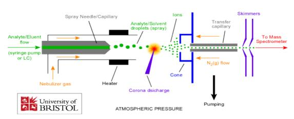
Fig 3 Mechanism of Atmospheric pressure chemical Ionization
