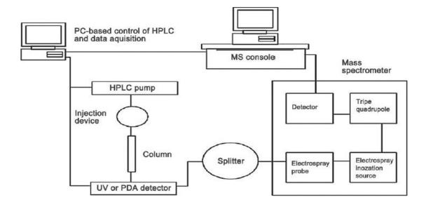
Fig.1 Schematic diagram of LCMS instrument
