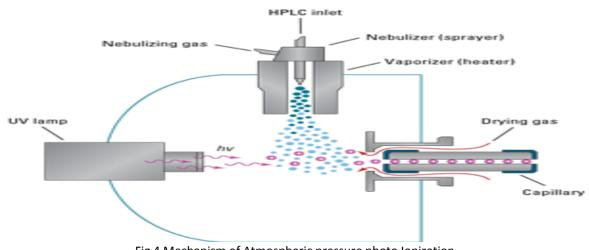
Fig 4 Mechanism of Atmospheric pressure photo Ionization
