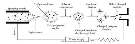
Fig 2 Mechanism of Electro spray ionization
