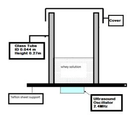
Figure 1: Experimental setup, ultrasound reactor.
