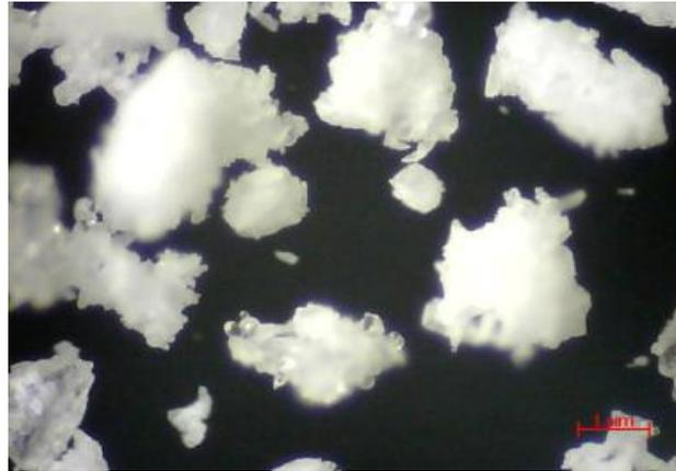
Fig. 1. The structure of granulate consisting lactose in amount of 5 %, 10 %, 25 %
