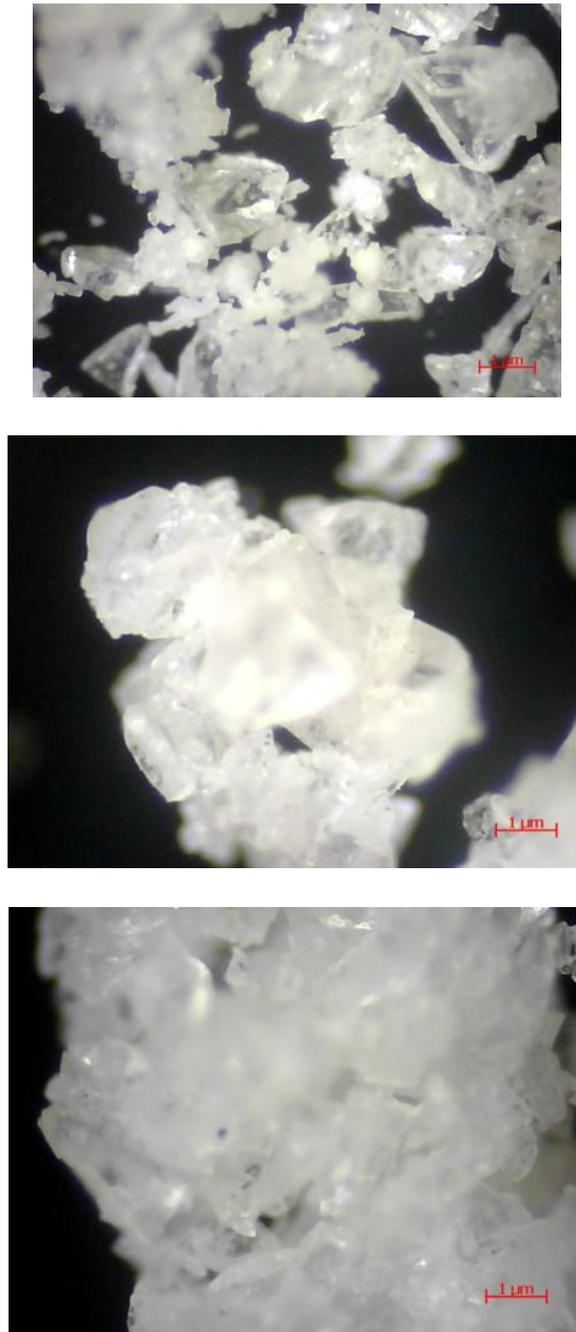
**Fig. 3. The structure of granulate consisting lactose and MCC in amount of 5 %, 10 %, 15 %**
