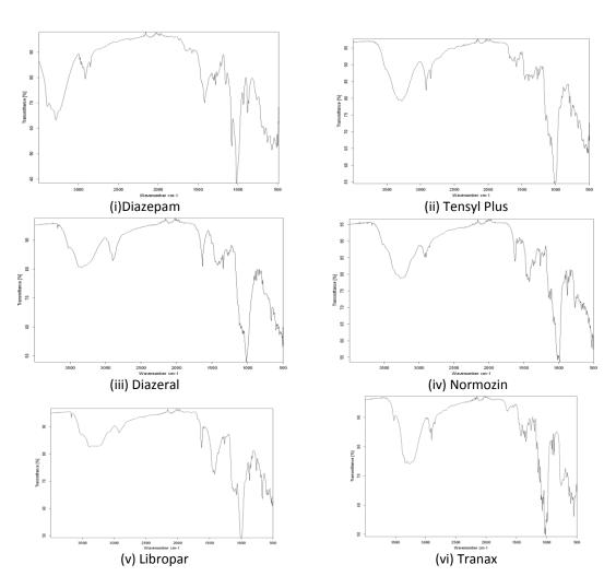
Fig. 2: FTIR-ATR spectrum of (i) Diazepam, (ii) Tensyn Plus, (iii) Diazeral, (iv) Normozin, (v) Libropar and (iv) Tranax.
