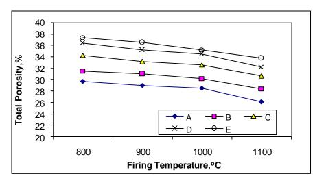
Figure (3) Effect of firing temperature from 800 °C up to 1100°C on the Total Porosity of tested samples having 0-10% of cement dust
