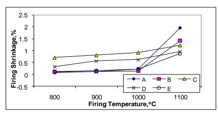
Figure (1) Effect of firing temperature from 800°C up to 1100°C on the shrinkage of tested samples having 0-10% of cement dust
