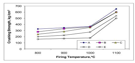
Figure (4) Effect of firing temperature from 800 °C up to 1100°C on the Crushing Strength of tested samples having 0-10% of cement dust
