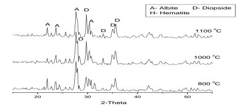
Figure (6): XRD patterns of the sample containing 5% cement dust fired at different temperatures.
