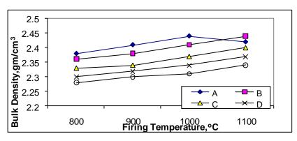
Figure (2) Effect of firing temperature from 800°C up to 1100°C on the bulk density of tested samples having 0-10% of cement dust
