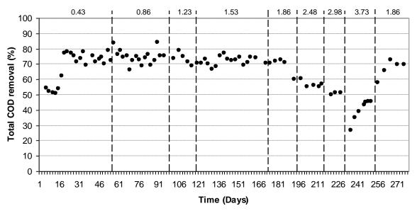
Figure 2. Total COD reduction (%) of the UASR treating pharmaceutical wastewater
