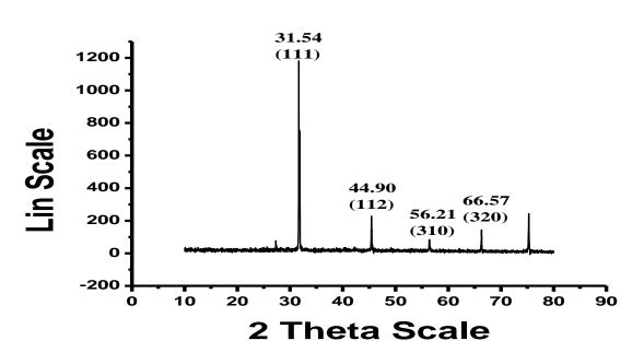
Fig. 3: XRD Graph confirming the presence of ZrO Nanoparticles
