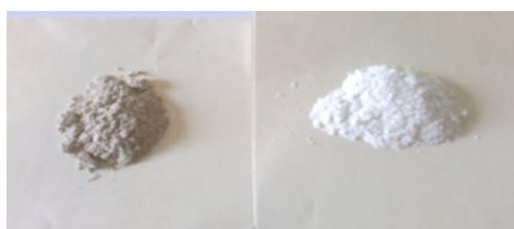
Figure 2: Image of the purified struvite after precipitation from sewage waste water and dark residual soids.
