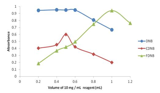
Figure 4: Effect of volume of reagents on the absorbance intensity of the reaction products of 10 μg/mL NAB with 10 mg/mL DNB, 120 μg/mL NAB with 10 mg/mL CDNB and 50 μg/mL NAB with 1% v/v FDNB.
