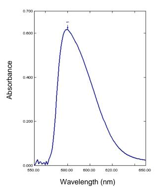
Figure 1: Absorption spectrum of the reaction product of 6  $\mu$ g/mL NAB with DNB in DMF.
