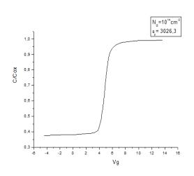
Figure No. 3: Total Capacitance of the Structure with Blood in Place of Airgap.
