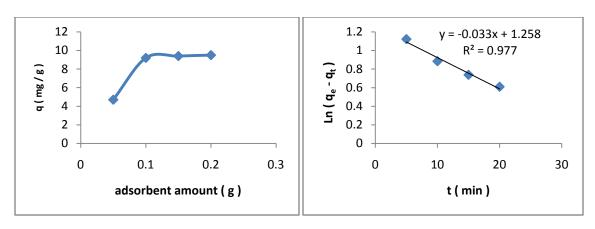
Fig6. Effect of adsorbent amount on the adsorption
