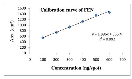
Fig. 6: Calibration curve of Fenofibrate
