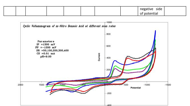
Fig: 2 Cyclic Voltammogram of *m*-Nitro Benzoic Acid at 9.0 pH
