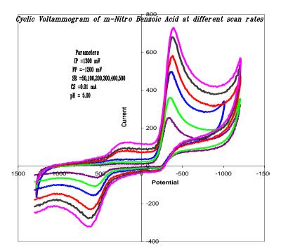
Fig: 1 Cyclic Voltammogram of *m*-Nitro Benzoic Acid at 5.0 pH
