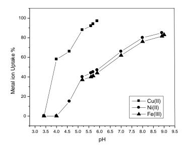
Figure-5: Uptake of Cu<sup>2+</sup>, Ni<sup>2+</sup>, and Fe<sup>3+</sup> ions by the resin immobilised on silica gel with pH variation.
