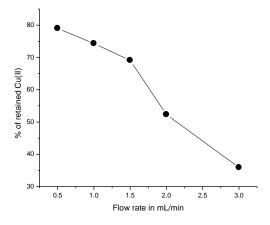
Figure-7: Study of adsorption behaviour in column operation with variation of flow rate of metal ion solution
