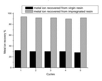
Figure-8: Comparison of elution of metal ion from virgin resin and impregnated resin.
