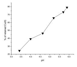
Figure-6: Study of adsorption behaviour in column operation with variation of pH of the medium
