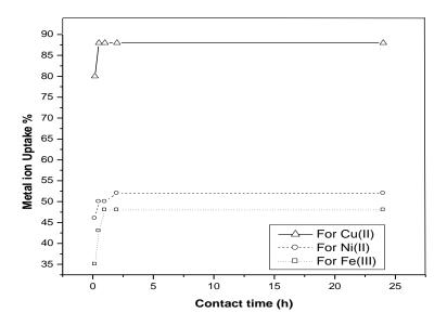
Figure – 3: Uptake of Cu<sup>2+</sup>, Ni<sup>2+</sup>, and Fe<sup>3+</sup> ions by the resin immobilised on silica gel with increasing contact time.
