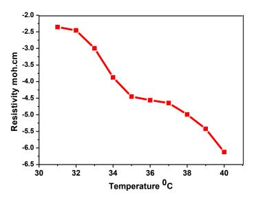
Fig 7: Resistivity Variation of Pseudomonas aeruginosa and MgFe<sub>2</sub>O<sub>4</sub> with reciprocal operating temperature.
