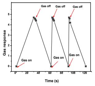
Fig 11: Response and recovery of the sensors.
