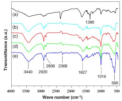
Fig 5: FT-IR spectra of the MgFe<sub>2</sub>O<sub>4</sub> composite samples calcined in air for 4 h at different temperatures. (a)  $-180^{\circ}$ C, (b)  $-500^{\circ}$ C, (c)  $-600^{\circ}$ C, (d)  $-700^{\circ}$ C, and (e)  $-800^{\circ}$ C.
