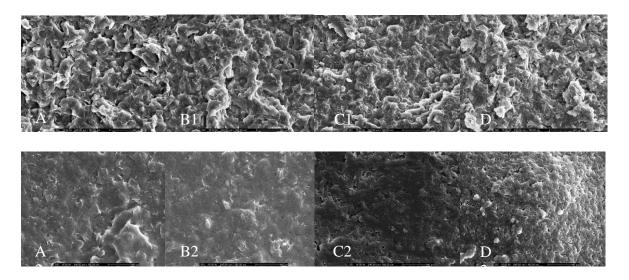
Fig. 1 Morphology of SW:Lut at various ratios 3:7 (A), 4:6 (B), 6:4(C), 7:3 (D) at magnification of 500X. The No. 1 was the surface of the bases and No. 2 was the cross-section of the bases.
