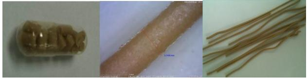
Fig. 2 The obtained extrudates (A) with close up surface (B) and filled in the capsule No. 1(C)
