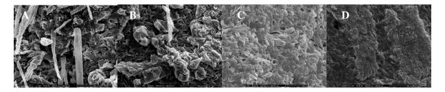
Fig. 4 SEM image of 10% (A), 20% (B), 30% (C) and 40% w/w (D) Ibu-loaded 7:3 Sw:Lut extrudates at magnification of 500.
