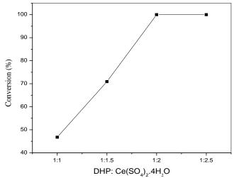
Figure 2 - Effect of amount of Ce (SO<sub>4</sub>)<sub>2</sub>,4H<sub>2</sub>O on the conversion DHP to pyridine
