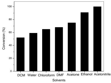
Figure 1 - Effect of reaction medium (solvent) on the conversion DHP to pyridine
