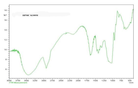
Figure No: 04 FTIR Spectral studies for HPMC K100M
