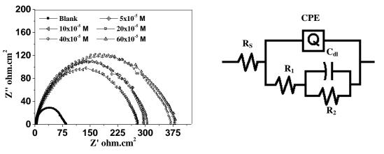
Fig. 8. Nyquist plot, together with the equivalent circuit used to simulate the impedance data, recorded for carbon steel in 1.0 M HCl solution in absence and presence of different concentrations of drug inhibitor.
