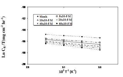
Fig. 6. Transition state plots for carbon steel in 1.0 M HCl solution in the absence and presence of different concentrations of the inhibitor
