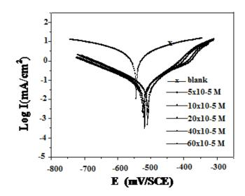
Fig 7. Polarization curves for carbon steel in 1.0 M HCl in absence and presence of different concentrations of drug inhibitor.
