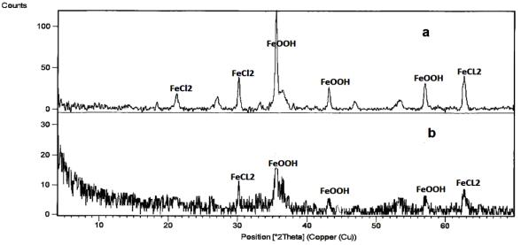
Fig.9- XRD patterns of corrosion products formed on the surface of carbon steel, (a) After 48 h immersion in 1.0 M HCl, (b) After immersion in 1.0 HCl containing 60x 10<sup>-5</sup> M inhibitor.
