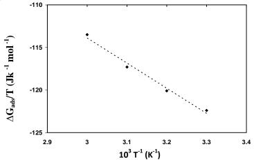
Fig. 4. Variation of  $\Delta G^{o}_{ads}/T$  versus T on carbon steel in 1.0 M HCl containing drug inhibitor.
