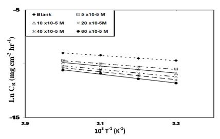
Fig.5. Arrhenius plots for carbon steel in 1.0 M HCl solution with different concentrations of the inhibitor.
