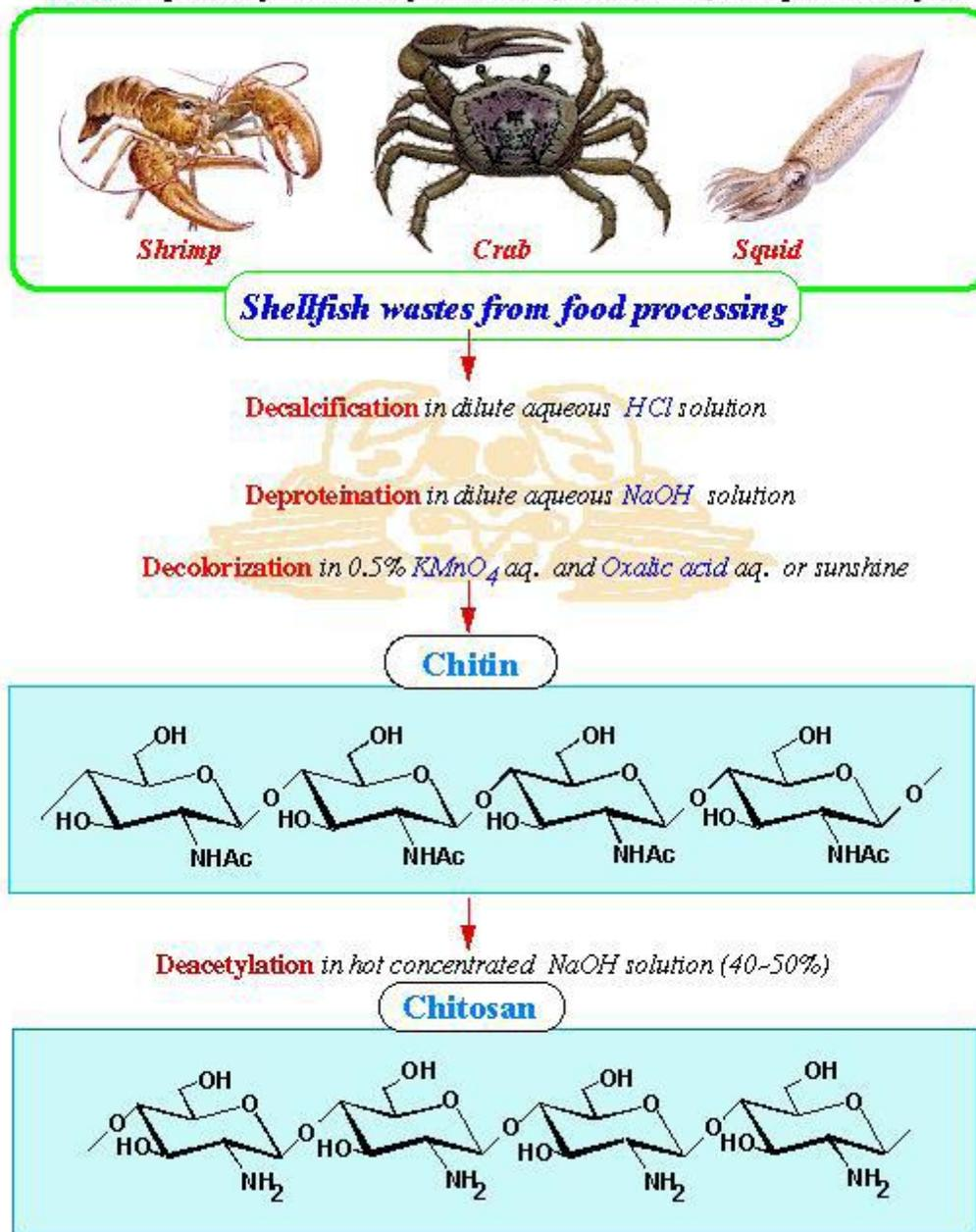
Fig. 2. Preparation of chitin and chitosan
