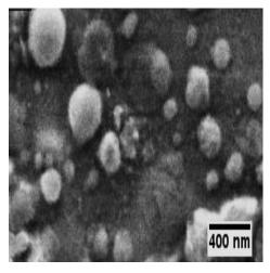
Fig.1: SEM Study of Chitosan TPP Nanoparticles
