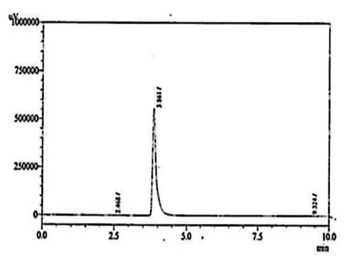
Figure 1: HPLC profile of metronidazole from blood plasma.
