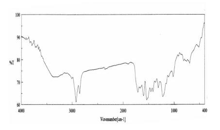
Fig. 2 IR Spectrum of cardanol-formaldehyde resin
