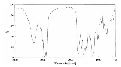
Fig. 3 IR Spectrum of rigid polyurethane
