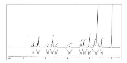
Fig. 1 <sup>1</sup>H–NMR Spectrum of cardanol-formaldehyde resin
